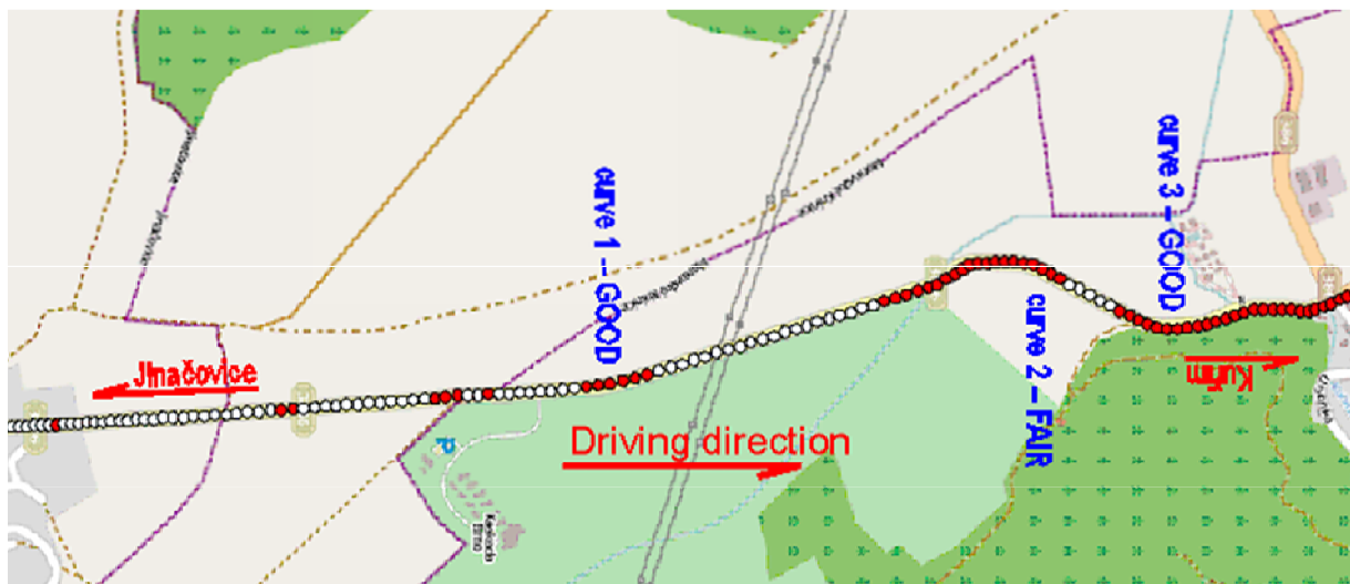
Fig. 4. Assessment of consistency of three curves of the route in question
